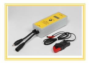
The ALS Current Meter is a hand held, digital meter designed to indicate current by direct measurement, or by using a current clamp, to within ± 1% of the correct value. This can be achieved even when measuring waveforms generated by Constant Current Regulators (CCR) with crest factors not exceeding 3.2, the maximum allowed in IEC61822. This small, portable instrument can also be used to safely set up the output from a CCR. The Current Meter is also included in the ALS sign Maintenance Kt.
